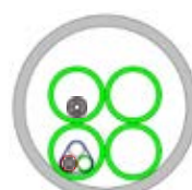
Existing Microduct in Duct
